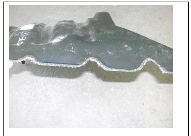
Figure 16: Liner looks like this after trimming
